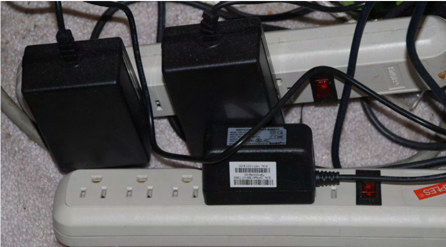
Figure 1- typical SC power strip with multiple "wall wart" DC power supplies attached
